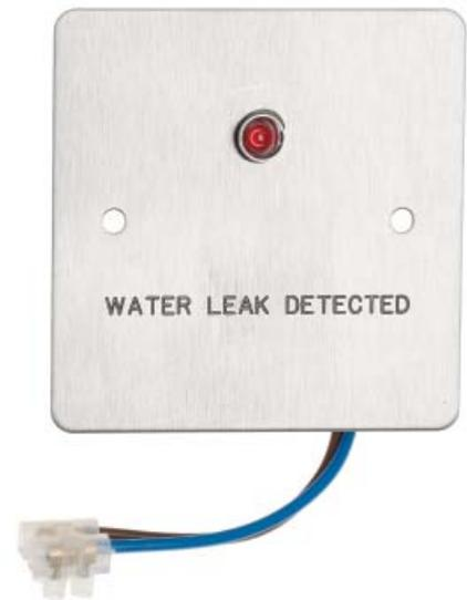
The AT-IWP is an Indicator Warning Plate used to provide a remote alarm signal from a TraceTek or AquiTron leak detection panel. The AT-IWP incorporates a red LED indication when an alarm is present. Can be supplied with either a 230Vac or 24Vac LED, please specify when ordering.
